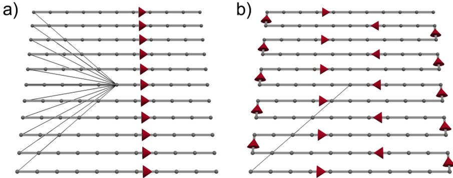
Figure 3.4. Trajectories through  $k$ -space for the acquisition of a slice. a) acquiring a slice line-by-line; b) acquiring a slice with EPI readout.
