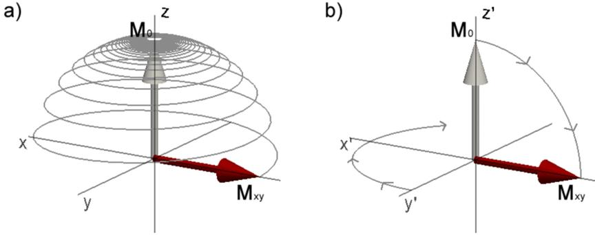
Figure 3.1. Magnetization during excitation with an RF pulse with 90° flip angle. a) in the laboratory frame of reference the magnetization  $M_0$  oscillates from its equilibrium position on the z-axis to the transverse plane resulting in a transverse magnetization  $M_{xy}$ . b) shows the same process as in a), but seen from the rotating frame of reference rotating about z at the resonance frequency.
