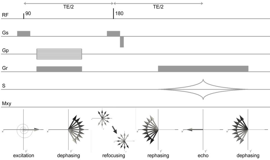
Figure 3.2. Sequence diagram and phase evolution in the transverse plane for the basic spin echo sequence. Gs, Gp and Gr are the gradients applied in the slice, phase and read direction, respectively.
