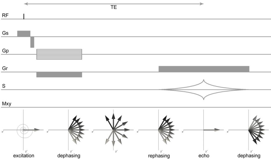
Figure 3.3. Sequence diagram and phase evolution in the transverse plane for the basic gradient echo sequence. Gs, Gp, Gr are the gradient applied in the slice, phase and read direction, respectively.
